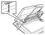
Attach the KX-DT301 to your unit with the screws (included with KX-DT301).
